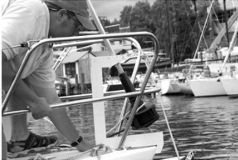
Beyond class rule compliance, the template provides a good tool for making setup of the rig accurate and repeatable. One of the major sail makers has commented that headstay setup is the single most important rig adjustment we can make. This is because the design program that makes the sail design has built in a certain amount of headstay sag when computing the shape. More or less sag affects the idea shape of the sail.
